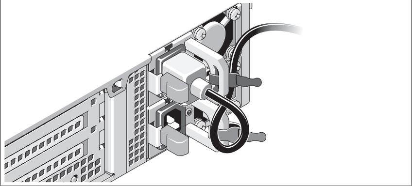
Bend the system power cable into a loop as shown in the illustration and secure the cable to the bracket using the provided strap. Plug the other end of the power cable into a grounded electrical outlet or a separate power source such as an uninterruptible power supply (UPS) or a power distribution unit (PDU).
